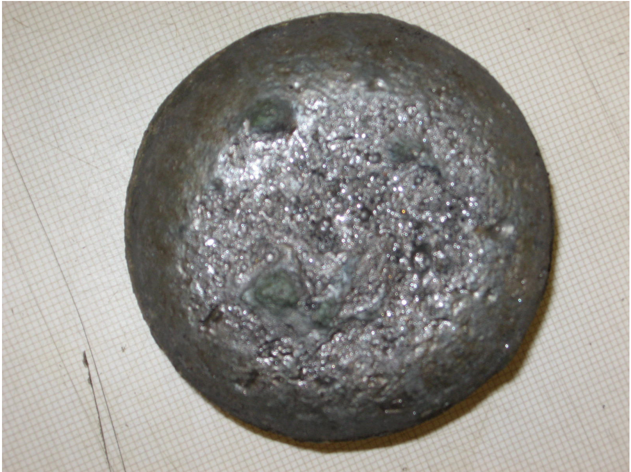
Figure 5 - Charge Chrome Puck after melt
